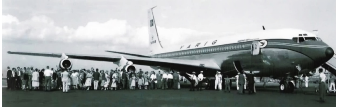
Figure 5: Boeing 707-441, Rolls-Royce Conway MK 508 turbofan engine which enabled non-stop Rio-New York flights. On the fuselage, the VARIG logo with Futura typography and on the tail the national flag with the Icarus mark.
