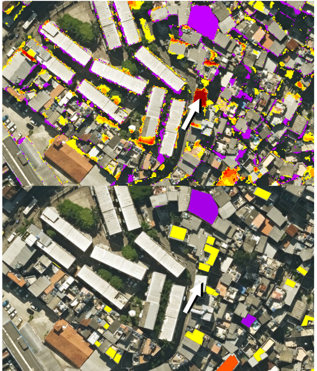
Figure 21: A comparison of change detection results using raster (top) and vector (bottom) data models for the period 2014–2019. The raster output shows edge noise due to minor planimetric shifts between surveys, while the vector output, derived from zonal statistics, omits a new building (see arrow) constructed after 2019.
