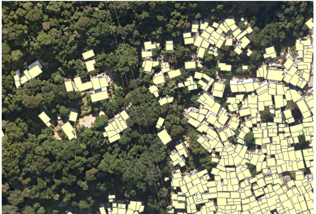
Figure 2: Building polygons derived from the 2013 photogrammetric restitution
