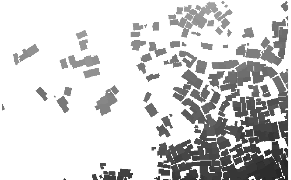
Figure 10: Extruded building footprints according to roof altitude
