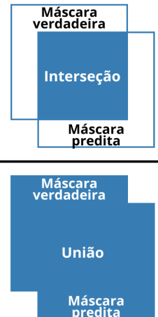
Figure 12: Illustration of the IoU (Intersection over Union) concept, showing the intersection area between the true mask and the predicted mask in relation to the union area of both.
